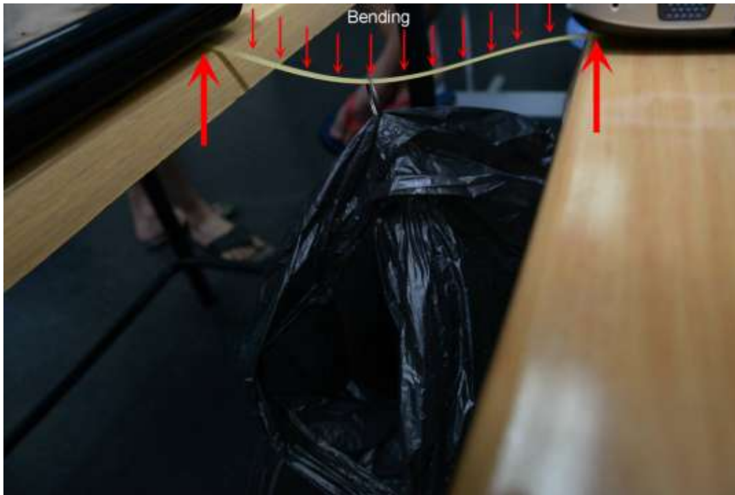
PICTURE 4.1.1 The loads (and reactions) bend the fettuccine and try to shear through it
